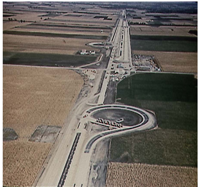
AASHO Road Test, still the basis of design used by many agencies until the Mechanistic-Empirical Design Guide is adopted by AASHTO.
