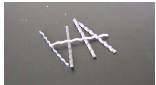
Some steel fibers have hooked ends and are collected in bundles that break apart during mixing (above) while others may be crimped in shape and unattached (below).
