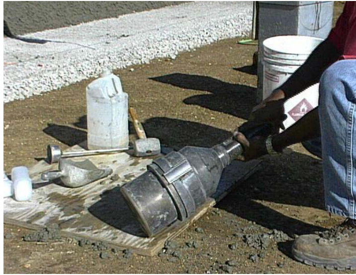
Figure 2. Traditional apparatus for measuring air content using the volumetric method (roll-a-meter).
