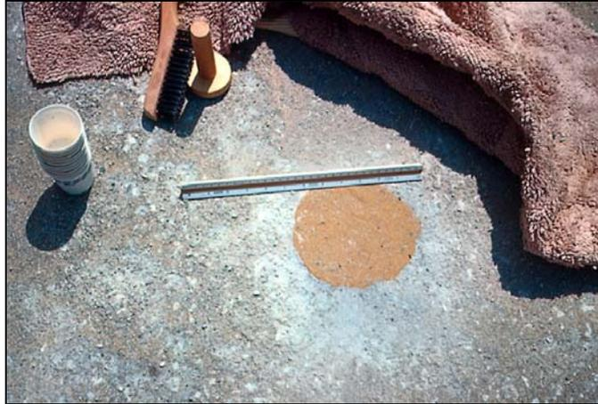
Figure 3. Using sand patch method (ASTM E 965) to test for surface texture depth.
