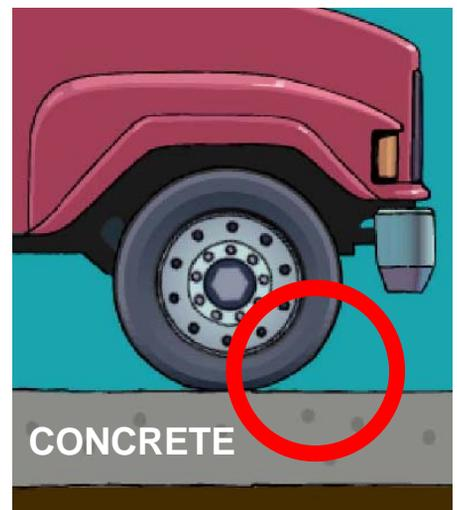
*The rigid surface undergoes negligible deflection ... no wasted energy means no wasted fuel.*
